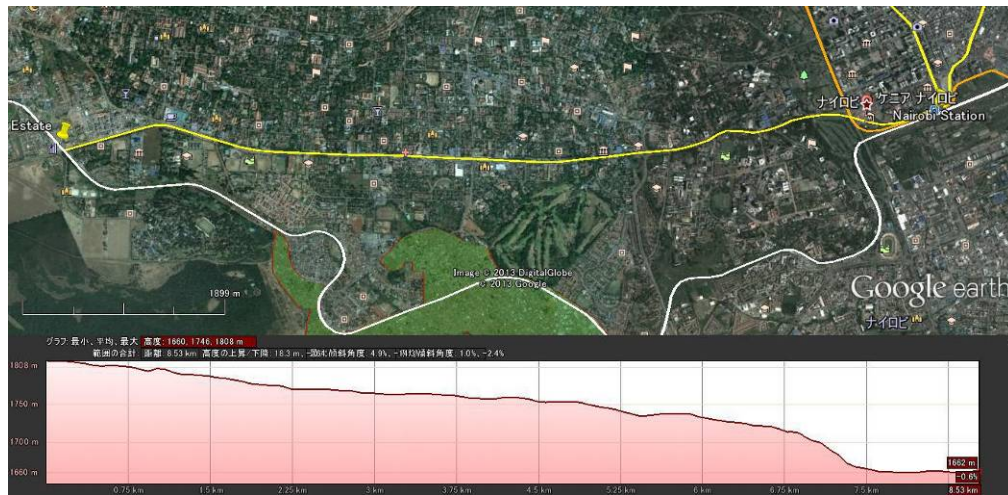
Figure 4.2.11 Horizontal and Vertical Alignments of MRT on Ngong Road
